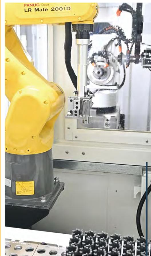
*Robot Loader allows us to load annular cutters automatically.*
